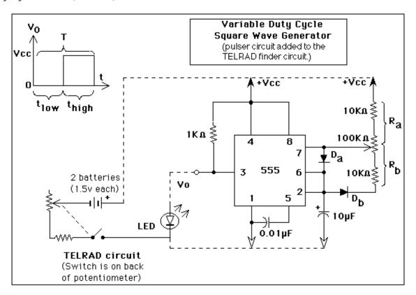
To use with the Telrad, connect Vcc to the battery positive side and ground to the battery negative side. You may do this through the switch already installed in the Telrad to control power. The Telrad's LED lead going to the positive side of the batttery is
